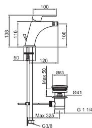
Single lever bidet mixer with Ø25 mm ceramic cartridge, 3/8" connections, 370 mm. long hoses, "luxe" pop-up waste set 1 1/4" and "plus" aerator. Flow rate (mixed water) 9.8 l/min. at 3 bar.
