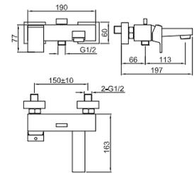
**1** Wall mounted exposed shower mixer with Ø35 mm ceramic cartridge and 1/2" connections. Centre distance 150 +/-10 mm. Flow rate (mixed water) 22,8 l/min. at 3 bar.
