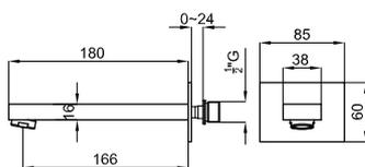
Concealed bath spout. "Clean" aerator. Flow rate (mixed water) 21 l/min. at 3 bar.
