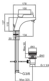
Single lever basin mixer with Ø28 mm ceramic cartridge, 3/8" connections, 370 mm. long hoses, "luxe" pop-up waste set 1 1/4" and "clean ECO" aerator. Flow rate (mixed water) 5 l/min. at 3 bar.
