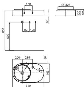
65 cm. wall hung basin with overflow and fixing kit 100041151 - N401150000.
