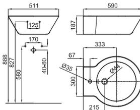
51 cm. wall hung basin with overflow. Fixing kit 100041225 - N421040000 included.
