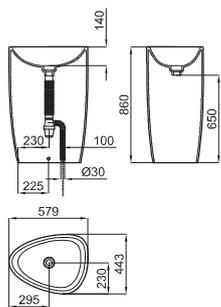
Floor standing basin without overflow. With flexi bottle trap floor outlet installation. Fixing kit 100041212 - N420150000 and pop-up waste with ceramic plug (installed in the basin).
