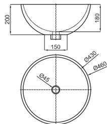
Ø46 cm. countertop basin without overflow. It's necessary to use a un-slotted clicker or freeflow grid basin waste.
