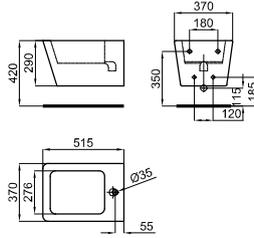
Wall-mounted bidet with concealed drain pipe-flush valve. It includes fasteners 100123732-N499816966. The 100046585-N499816802 concealed drain adapter is sold separately
