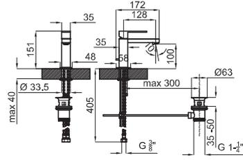
Single lever basin mixer in chrome (100038688 - N161010001) with colour insert 3/8". Ø25 mm, ceramic cartridge. Length of hoses 405 mm. With pop-up waste set 1 1/4". "Plus" aerator. Flow rate (mixed water) 10,5 l/min. at 3 bar.
