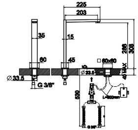
**1** Infra-red operated basin tap 3/8". Without pop-up waste. "Plus" aerator. Flow rate (mixed water) 10,5 l/min. at 3 bar.
