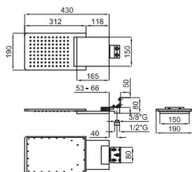
Rain+cascade shower head with 1/2" connectors. Flow rate rain: 12,3 l/min. at 3 bar and flow rate cascade: 8,80 l/min. at 3 bar.
