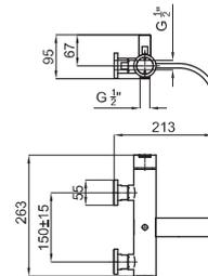
**1** Wall mounted exposed shower mixer with Ø35 mm ceramic cartridge and 1/2" connections. Centre distance 150 +/-15 mm. Flow rate (mixed water) 18,72 l/min. at 3 bar.
