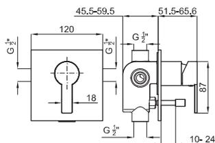
Single lever concealed shower valve with diverter 1/2". Ø35 mm ceramic cartridge Automatic diverter. Flow rate shower: 21,52 l/min. at 3 bar and flow rate bath: 22,34 l/min. at 3 bar.
