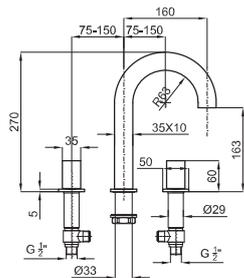
3 hole basin mixer with 1/2" connections. Ceramic disc valves (90°). Without aerator (incorporate flow-bracker). Flow rate (mixed water) 10,23 l/min. at 3 bar.
