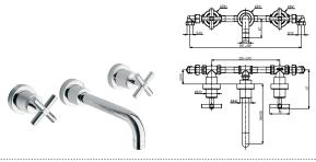
Wall mounted basin mixer with 1/2" connections. Ceramic disc valves (opening 90°). "Plus" aerator. Flow rate (mixed water) 13,06 l/min. at 3 bar.
