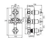
1 Concealed thermostatic 2 ways 1/2"-3/4" (see technical drawing) with wax thermostatic element. Manual diverter. Flow rate bath 26 l/min.at 3 bar and flow rate shower 13 l/min. at 3 bar. Built in nonreturn valve. Safety stop at 38°C.
