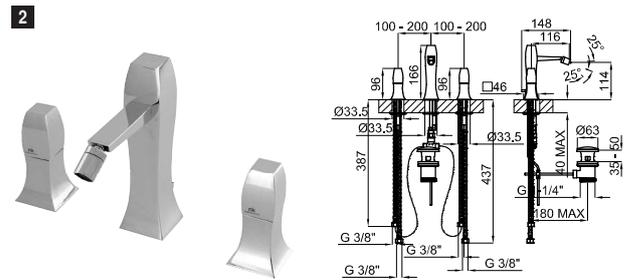
**1** Single lever bidet mixer with 3/8" connections. Ø25 mm.ceramic cartridge. Length of hoses 410 mm. With pop-up waste set 1 1/4". "Plus" aerator. Flow rate (mixed water) 9 l/min. at 3 bar.
