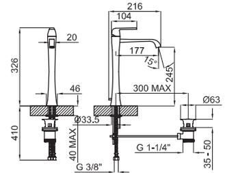
**1** Single lever basin mixer with 3/8" connections. Ø25 mm.ceramic cartridge. Connection 3/8". Length of hoses 410 mm. With pop-up waste set 1 1/4". "Plus" aerator. Flow rate (mixed water) 10,4 l/min. at 3 bar.
