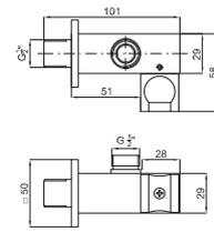
**1** Single function handshower . Flow rate (mixed water) 12 l/min. at 3 bar.
