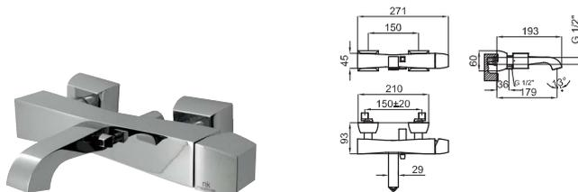
Wall mounted exposed bath shower mixer 1/2". Ø35 mm ceramic cartridge. Automatic diverter. "Plus" aerator. Centre distance 150 +/- 20 mm. Flow rate shower: 15,6 l/min. at 3 bar and flow rate bath: 20,3 l/min. at 3 bar.
