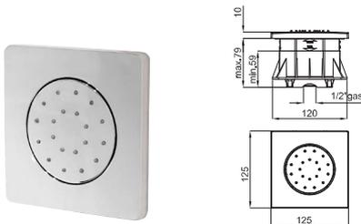
1/2" concealed body jet. Minimum flow rate required: 3,55 l/min. at 3 bar
