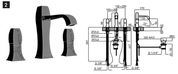
**1** 3 hole basin mixer with 3/8" connections. Ceramic disc valves (90°). Length of hoses 387 mm. With pop-up waste set 1 1/4". "Plus" aerator. Flow rate (mixed water) 10,5 l/min. at 3 bar.
