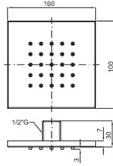
Wall mounted body jet 1/2". Minimum flow rate required: 4 l/min. at 3 bar
