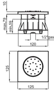
1/2" concealed body jet. Minimum flow rate required: 3,55 l/min. at 3 bar
