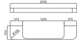
1 130 cm. wall hung basin with overflow. Fixing kit 100041225 - N421040000 included.
